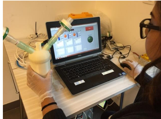
Experimental setup to test the breath sampler in a primary care facility in the Antwerp region
